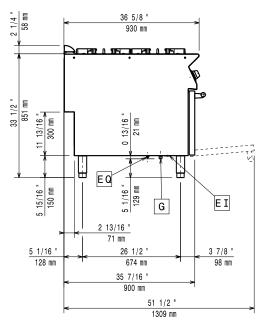
Electrical inlet (power) Gas connection
